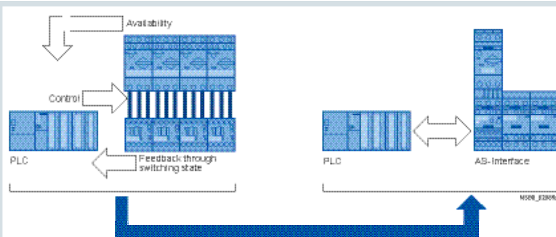
Signal transmission through AS-Interface
