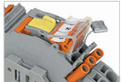
A lock-out seal can be used on the disconnect link in operating position I in connection with end and separator plate (2007-8893 or 2007-8894)
