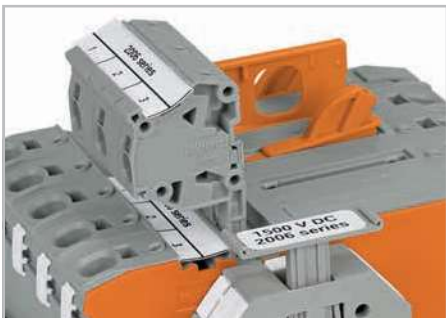
Alternatively, measurement can also be performed using TOPJOB® S connectors (2006-511) from terminal block 1 to 2. Spacer modules (2006-549) must be used to compensate for the 15 mm terminal block width.
