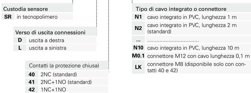
**Struttura codice azionatore singolo****SM A01N**
